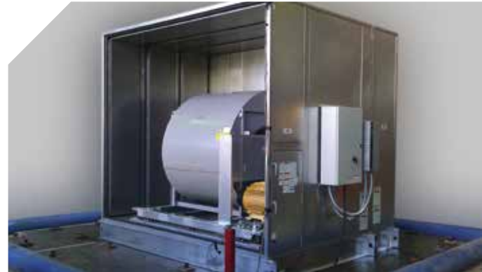
Vision air handler OSHPD pre-approval seismic testing on the University of California, Berkeley Pacific Earthquake Engineering Research (PEER) shake table.
